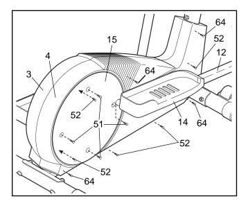
Next, remove the four Screws (51) from the right Pedal Disc (15), and slide the Pedal Disc off. Remove all Screws (52, 64) from the Right Side Shield (4), and remove the Right Side Shield. Remove all Screws (52) from the Left Side Shield (3) and remove the Left Side Shield.
